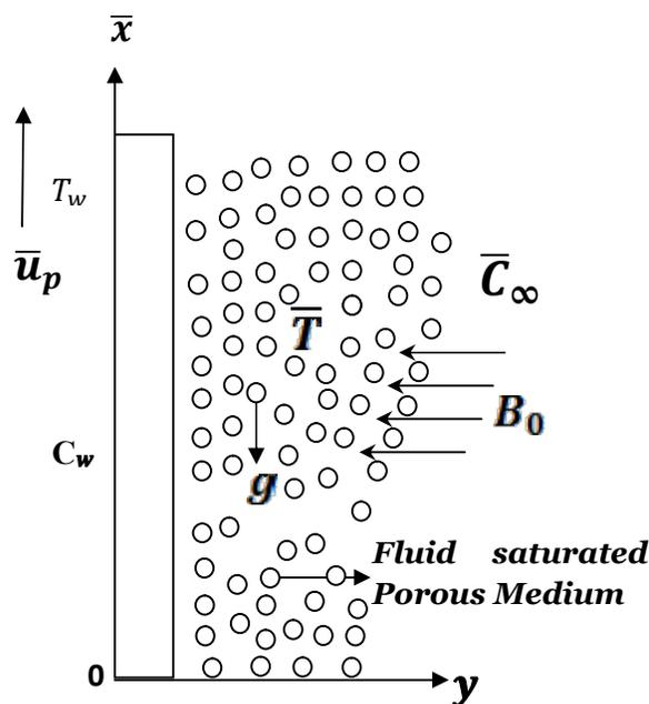
**Figure 7.2(a): Physical model and coordinate system**
