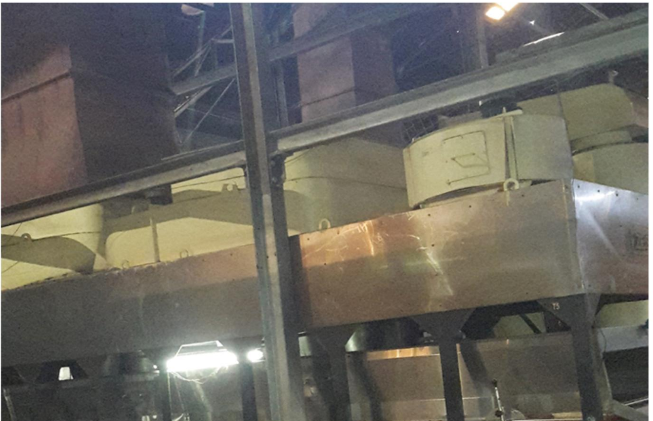
Drying of tea after fermentation inside a tea factory
